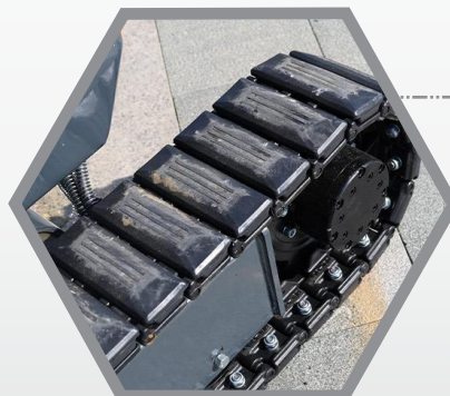
STANDARD STEEL TRACKS WITH RUBBER BLOCKS FOR DURABILITY & GROUND PROTECTION
