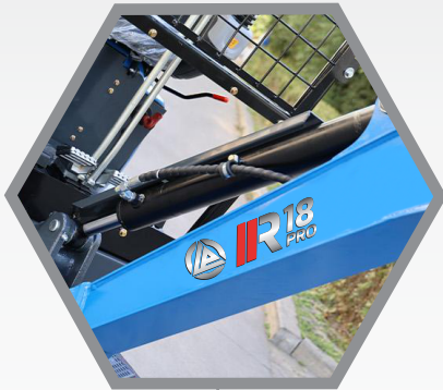
TOP MOUNTED BOOM CYLINDER WITH CYLINDER GUARD
