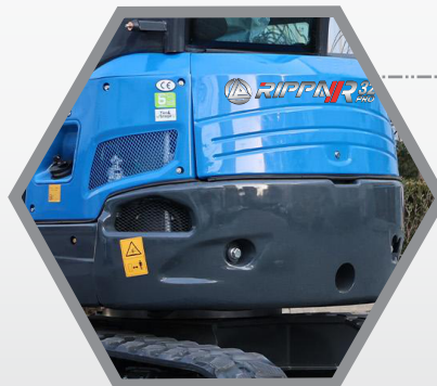
LARGE REAR COUNTER WEIGHT WITH ZERO TAIL SWING
